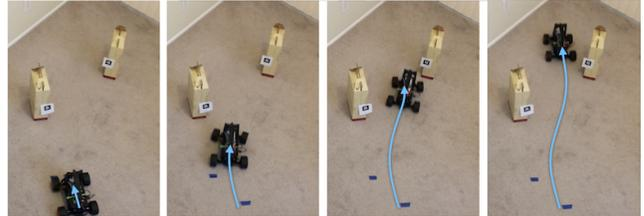
Fig. 1: A dynamically constrained mobile robot agent without prior knowledge of the environment successfully navigates a scene and avoids collision while equipped with only a monocular camera.
