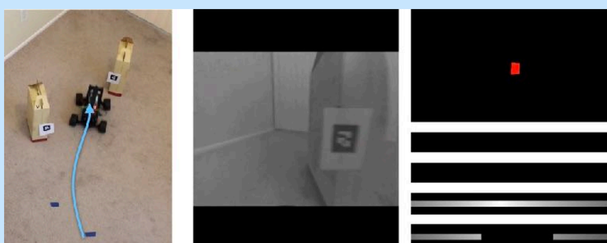
(c) As a result of avoiding the first obstacle, the agent approaches the second obstacle, which induces a different portion of the control set to become unavailable (bottom right).
