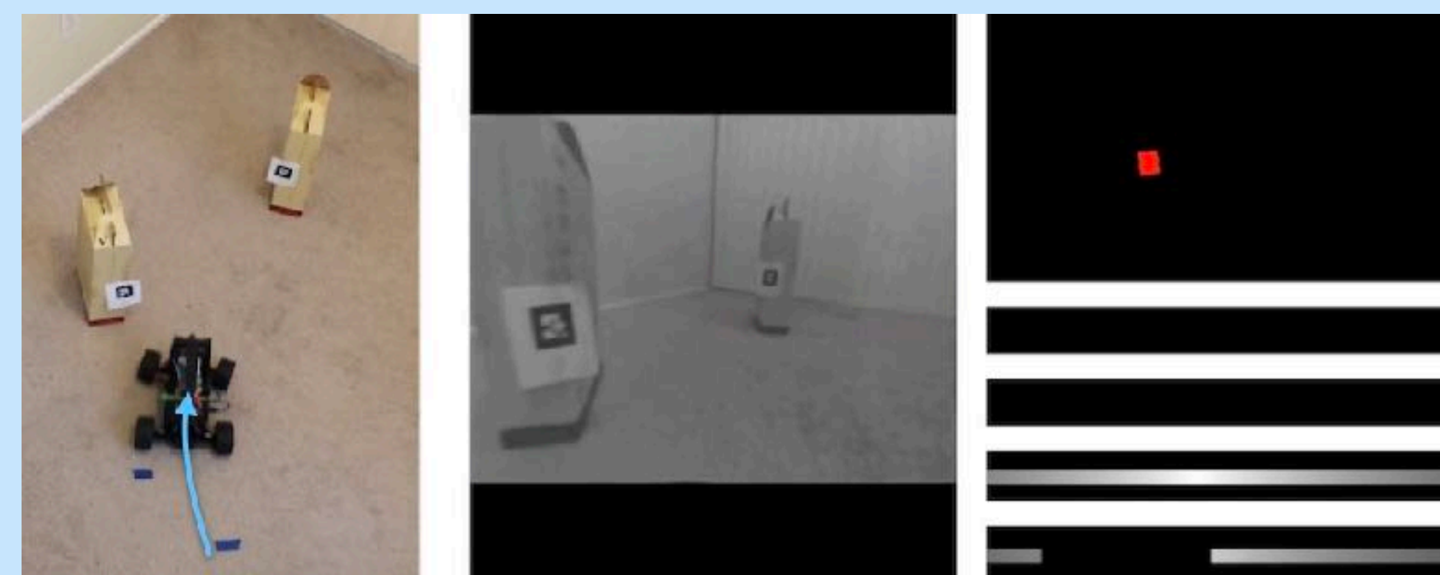
(b) Once the agent begins moving forward, the near obstacle induces an increasing negative potential region in the ISP field (top right). As the potential drops, the controls that steer the agent toward the obstacle are made unavailable (bottom right).
