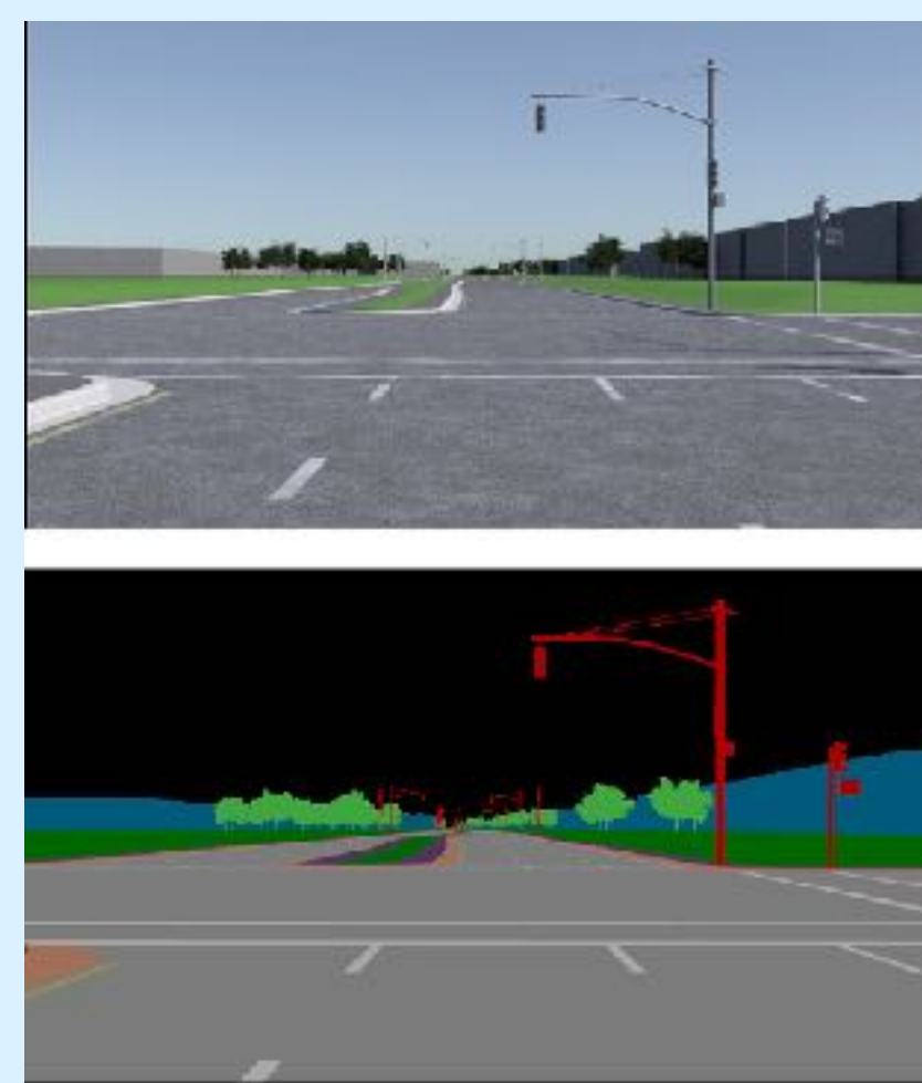
(a) Top: The raw camera image input. This image passes through a perception routine that can produce a segmentation. Bottom: The segmentation output of perception.
