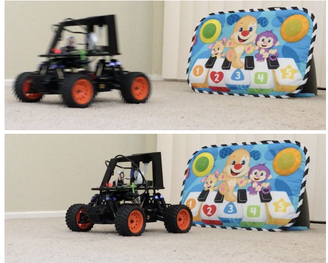
Fig. 1: Top: The Donkey Car encroaches on an object in its field of view. Bottom: The Donkey Car stopped at the point encroachment is detected. Video of this scenario at: https://youtu.be/QDZJRk6OJZQ
