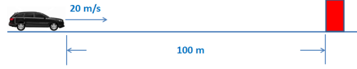
Fig. 2: Fixed Obstacle scenario. The car moves toward a fixed obstacle 100 m ahead with initial velocity 20 \text{ m/s} .
