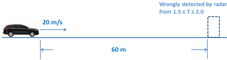
Fig. 5: False Positive scenario. The car starts at 20m/s with no obstacles detected. After 1.5 seconds, the car will wrongly detect an obstacle at position 60. This false positive period lasts for 0.5 seconds.
