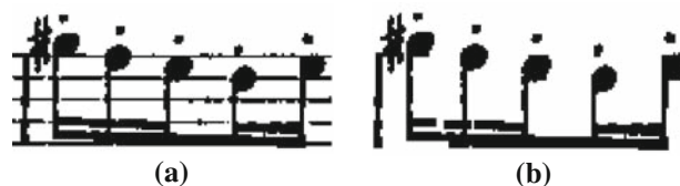
Fig. 2 An illustrative example of the staff line removal a music score with staff lines, b music score without staff lines
